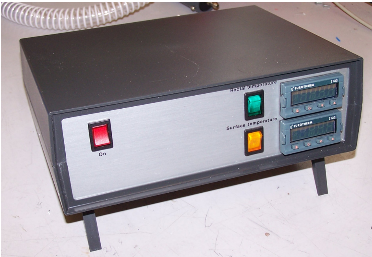
Figure 1. The control unit front panel. The neon indicators in the illuminated rocker switches enabling rectal and surface heating turn on when heating is required, as determined by thermocouple-sensed temperatures.
